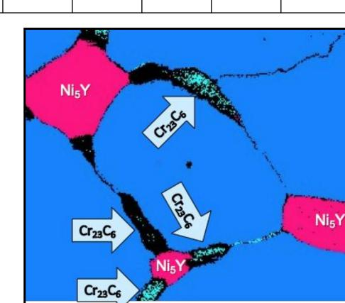
EDS and EBSD indicate the presence of M23C6 carbides, a Ni5Y phase, and a Ni-Cr matrix. Y and O were detected but not present in fine Y2O3 dispersoids. The presence of Si and decreased amount of Ti and Al indicate inadequate processing.
