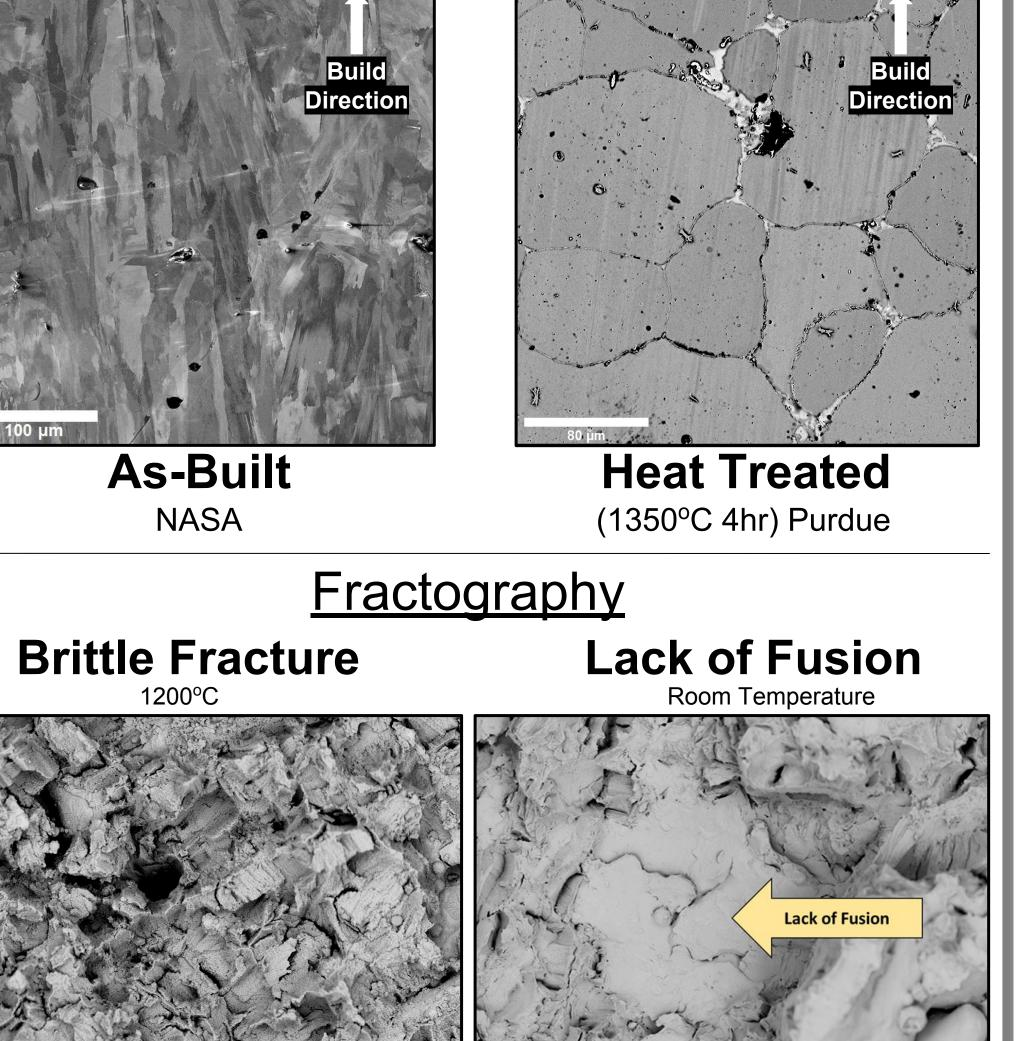
Comparison to literature suggests initial creep testing occurred in low creep exponent region where fracture by cavitation would be expected.
