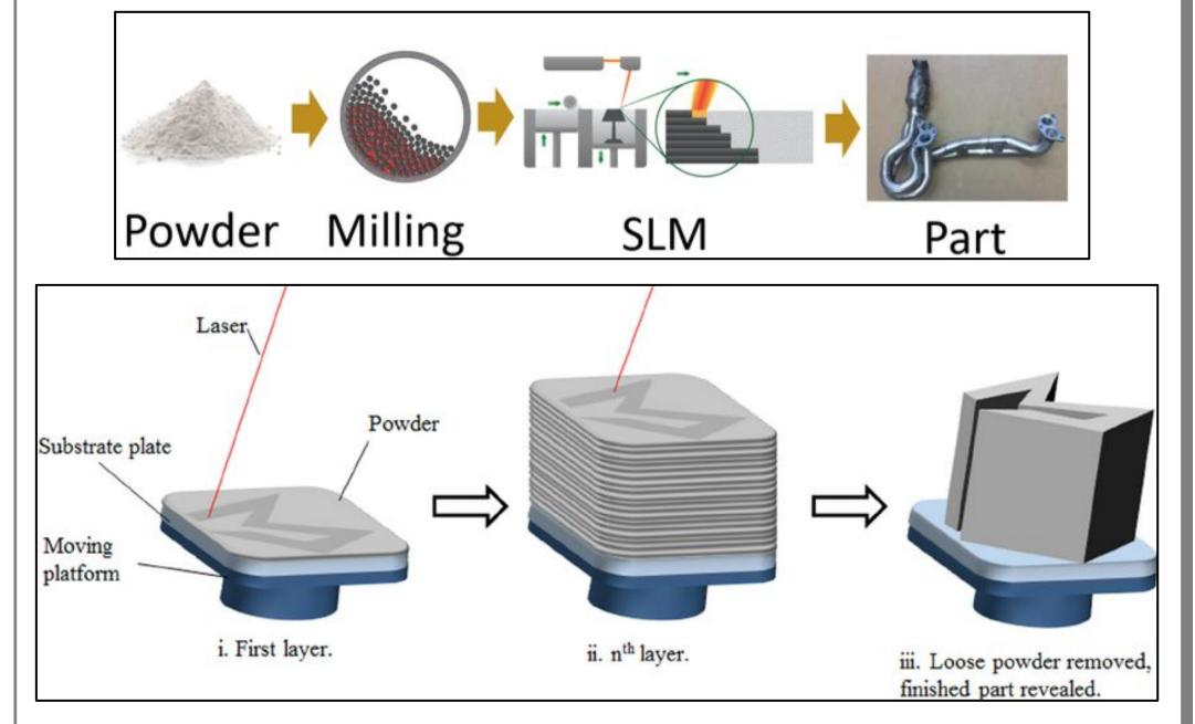
DMLM parts solidify directionally due to thermal gradients. Annealing can relieve resultant residual
